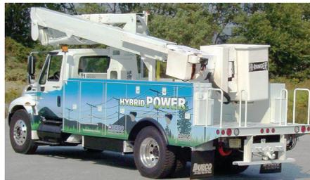
Odyne Corp. supplies hybrid components to partners who install them into medium and heavy-duty vehicles. Dueco installed the components into the aerial lift truck above. Now crews don't have to keep the engine running when they're operating the lift.
